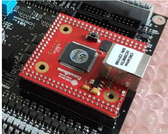
Figure 3, UC300ETH stack on UB1 breakout board.
